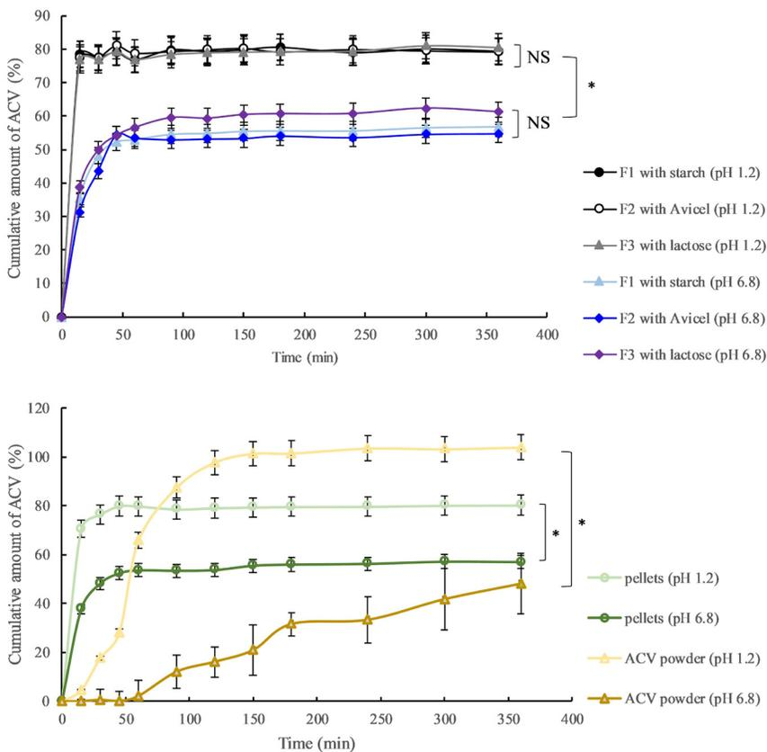
**Figure 4.** Dissolution profiles of ACV from MUPS tablets, pellets and capsules in different media, simulated gastric fluid (pH 1.2) vs. simulated intestinal fluid (pH 6.8) indicating significant (\*) and non-significant (NS) differences.
