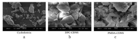
Figure 4. SEM image of a) Cyclodextrin b) Diphenyl Carbonate crosslinked NS c) Pyromellitic Anhydride crosslinked NS <sup>46</sup>
