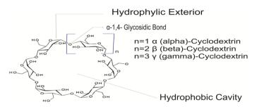
Figure 1. Dimensions and chemical structure for  $\alpha$ -,  $\beta$ - and  $\gamma$ -CD (n = 6, 7 and 8, respectively).
